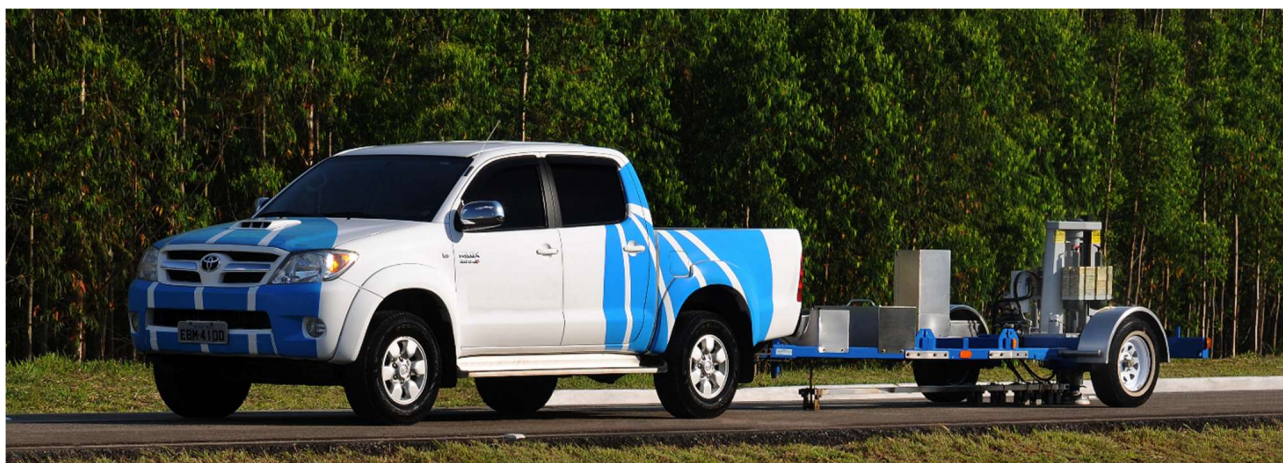
Figura 2 – Vista do Falling Weight Deflectometer Dynatest 8000.
